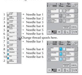
Since the thread colors on needle bars 2 and 3 will be used again after the thread spools are changed, they will not be replaced. However, different colors are assigned to the other needle bars.
